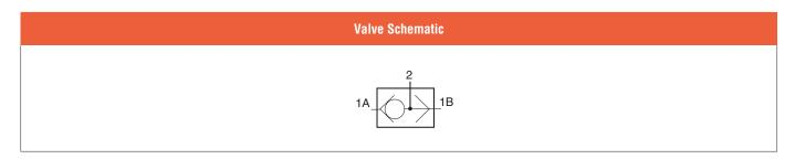
ROSS shuttle valves or double check valves have two inlets and one outlet. The first inlet to be pressurized is connected to the outlet, and the second inlet is then closed. Thus, a pneumatic device connected to the shuttle outlet can be operated by either of two control valves connected to the shuttle inlets. Automatically blocks one inlet passage when pressure is applied to the second inlet. Pressure to either inlet is channeled to one outlet port.
