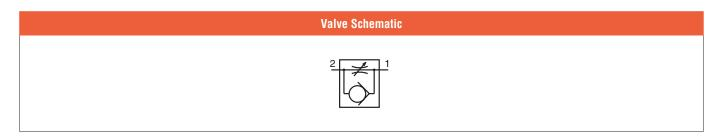
Selecting flow control valves with sufficient flow capacity is important so that they do not become the limiting factor in the cylinder control system. Full flow capacity should match that of the control valve to keep cylinder motion smooth and predictable in both directions.
