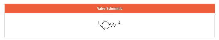
ROSS check valves are self-actuating and designed to provide free air flow in one direction, and to be closed to flow in the opposite direction.
